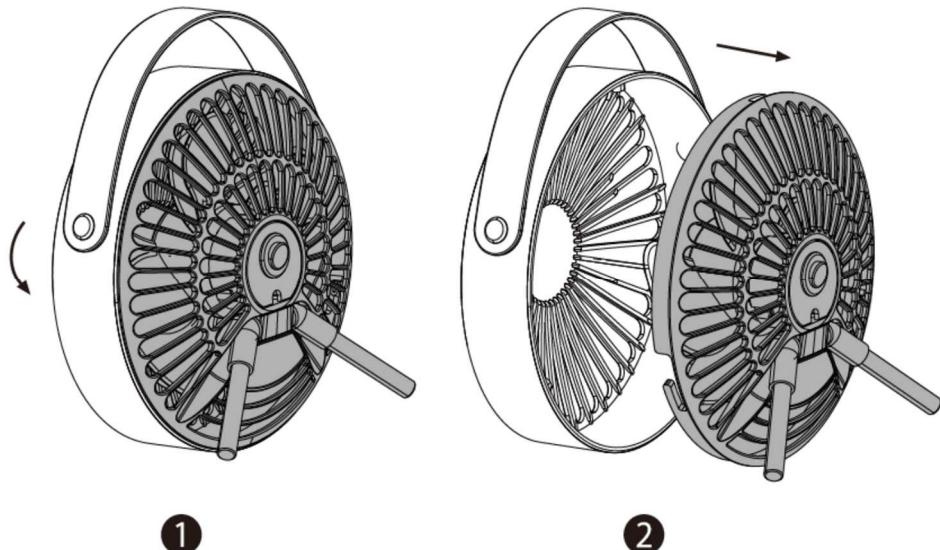
Clean the blades by using a soft dry cloth then close the grid by rotating it clockwise to assemble it with the rear grill:
