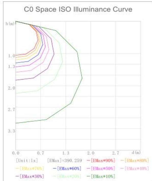
● Lux test diagram
