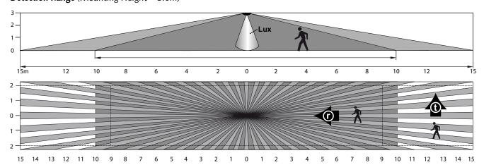
The detection range in side view (top) and top view (bottom).
