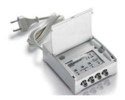
These amplifiers enables the user to amplify and distribute TV signals to every outlet, guaranteeing optimum signal level throughout the system. Compact and elegant design. Fully compatible with DTT signals in COFDM modulation. Metal Housing, fully shielded, with plastic cover and F connectors. Compatible with DTT signals in COFDM modulation.
