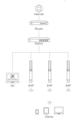
A DHCP server (typically a router) with DHCP function enabled is required to assign IP addresses to the EAPs and clients in your local network.
